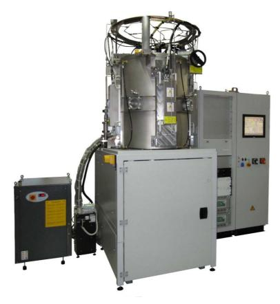
That new tool is able to deposit several different materials (metals, oxides, nitrides, carbides, diamond-like carbon), even gradient layers, onto flexible and rigid substrates from 5 rectangular sputter sources. It includes a radio frequency driven substrate drum and substrate heating.
